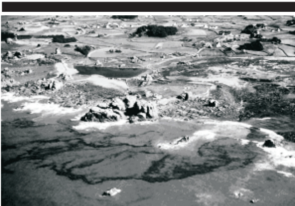
Figure 1. Example of Amoco Cadiz oil being held off rocky shore exposed to high wave activity, while tidal flat and gravel beach in background shows heavy oiling.
