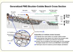
Subsurface oil sequestered in fine sediment beneat boulder/cobble "armor"
