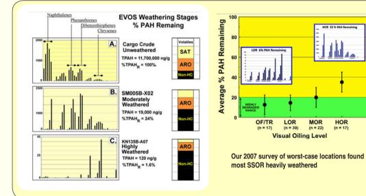
Because chemical weathering reduced total polycyclic aromatic hydrocarbon (PAH) concentrations, the toxicity of oil, as measured in standard amphipod bioassays done on sediment samples collected in 1990-1993, diminished after 1989.
