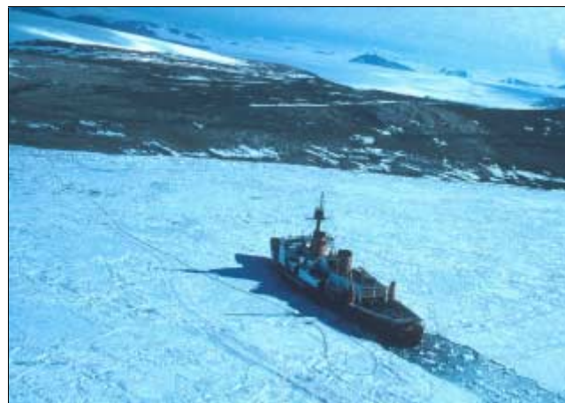
Figure 4. The USCG icebreaker Polar Seas offloading fuel to Marble Point. The offloading hose is visible to the left of the vessel.
