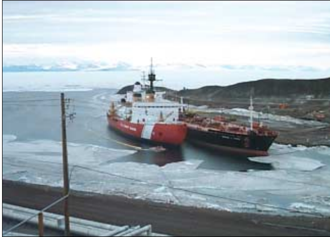
Figure 9. Boom deployment around USCG icebreaker and offloading tanker at McMurdo Station.
