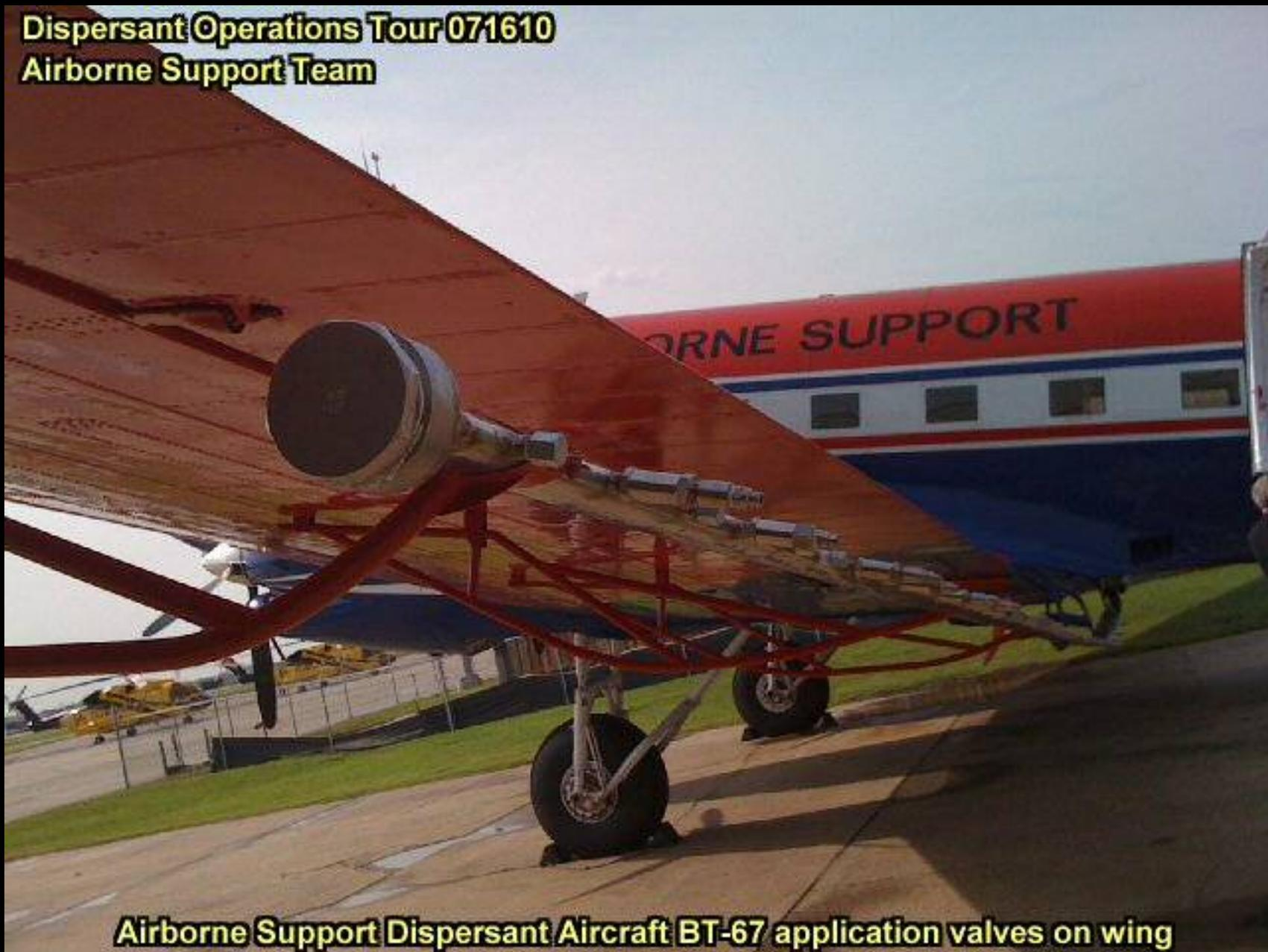
**Airborne Support Dispersant Aircraft BT-67 application valves on wing**
